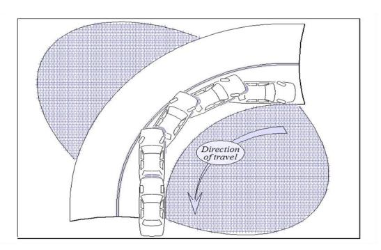
Rear wheel cheat When driving forward, the rear wheels will take a path inside that of the front wheels when the vehicle is turning. The sharper the turn, the greater the <u>rear wheel cheat.</u>
